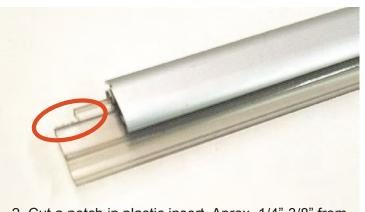
2. Cut a notch in plastic insert. Aprox. 1/4"-3/8" from edge. Do not cut below where clamp hinges. You can use a fine toothed saw, diagonal cutters or razor blade to complete this task.
